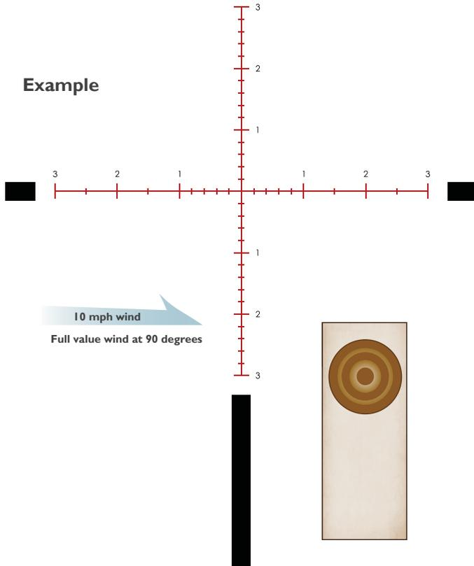
Using 3 mrad drop line at 500 yards, 2 mrad correction for 10 mph wind.
