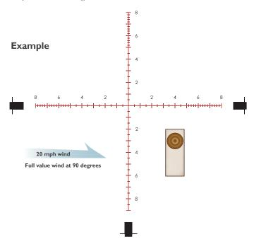
Using 3 mrad drop line at 500 yards, 4 mrad correction for 20 mph wind.
