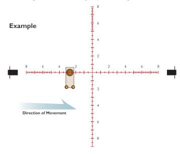
2.74 mrad correction for a target moving at 3 mph at 800 yards. No wind. Total bullet time of flight from trigger pull is 1.5 seconds during which the target travels 6.6 feet. Elevation already dialed into turret.
