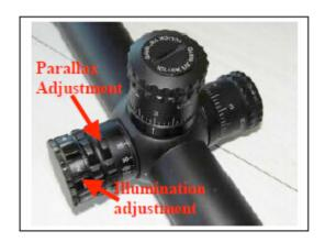
Figure 3: Adjustment of parallax to the distance of your target.
