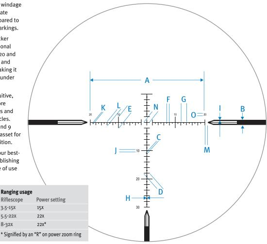
Image above shows the MOAR™ reticle used in 3.5-15x NXS riflescopes. It has 30 MOA below the centerline. MOAR™ reticles in 5.5-22x and 8-32x NXS models have 20 MOA below the centerline.
