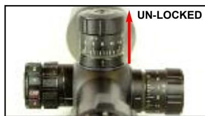
When a satisfactory zero is achieved, the turrets can be reset. To do this, simply loosen the hex screw on the top of the turrets and then pull the turrets up to their furthest extent. The turrets will then rotate without clicking. Adjust to the '0' zero point, push the turrets down to locate into the locked position and re-tighten the hex screw.
