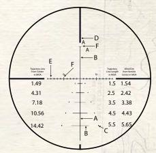
All Subtensions in MOA at 15X magnification. When modifying for 10X, leave all actual reticle dimensions the same except the Trajectory bar and wind spacing which must maintain it's MOA values as shown at 15X
