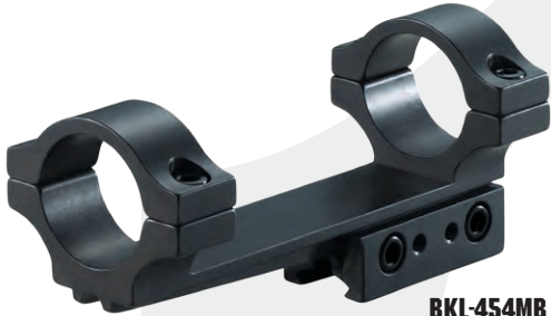
BKL-454MB 4" LONG CANTILEVER MOUNT WITH 1-5/8" CLAMPING LENGTH MATTE BLACK
