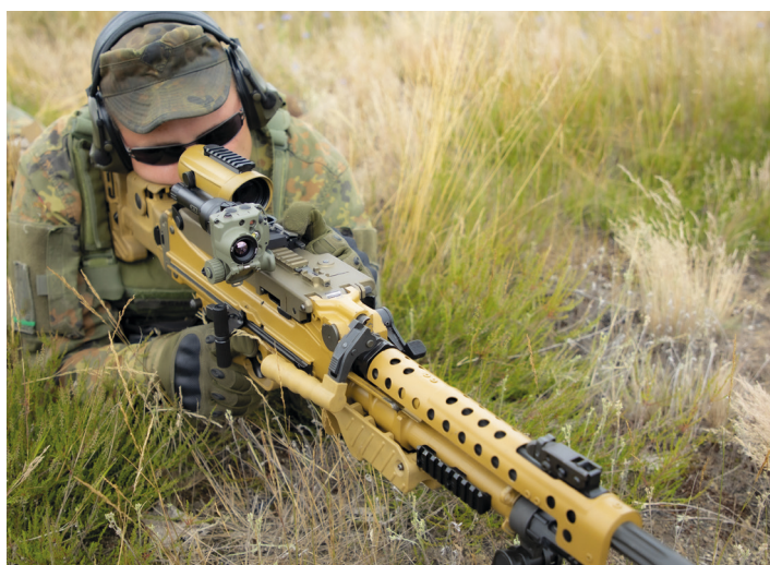
TILO-6MA folded down in front of a scope. (We recommend a maximum magnification of 2x).
